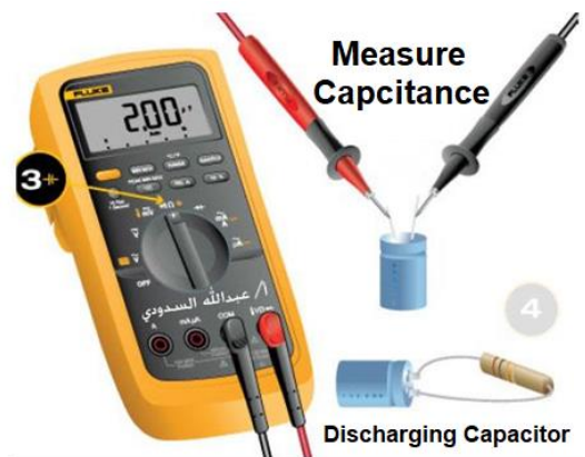
Capacitor measuring and
